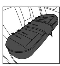
Insert the chuck of the seat cover into the gap of the seat connection.
