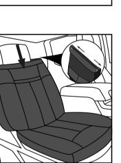
First open zipper on top of front seat cover, then put the cover into the seat as shown in diagram.
