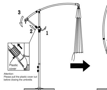
Step 1: Pull the button out. Step 2: Pull the plastic cover out. Step 3: Pull back pole to the end.
