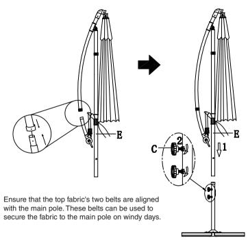
Please note: To insert the main frame, first, loosen Screws C as much as possible.
