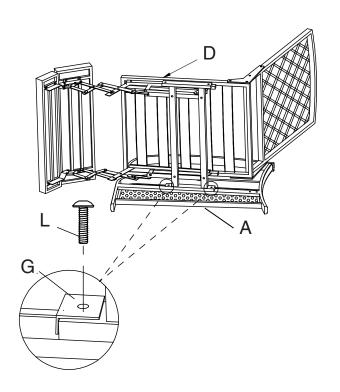
3. Connect Armrest (Part B) to Seat (Part D) using Washer (Part G) and Screws (J) as shown in the
