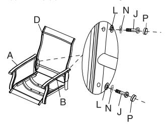
1. Connect the Right Arm (Part A) and Left Arm (Part B) to the Seat (Part C) using Bolt (J), Spring Washer (N), Washer (L), and Cap (P) as shown in the diagram.
