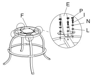
3. Attach Leg (Part E) and Leg Connector (Part G) using Bolt (K), Spring Washer (N), Washer (L), and Cap (P) as shown in the diagram.
