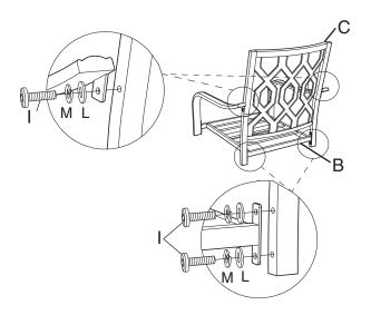
1. Connect the Right Arm (Part A1) and Left Arm (Part A2) to the Seat (Part B) using Bolt (I), Spring Washer (M), Washer (L) as shown in the diagram.
