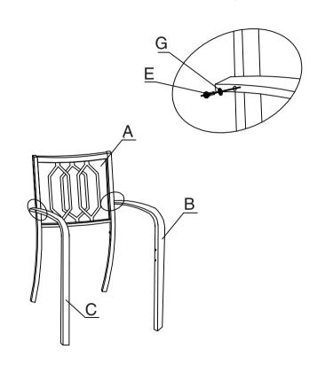
Connect Seat Part (D) with Back and Legs Part (A&B&C) using Screws (F) and Washer (G) as shown in diagram.
