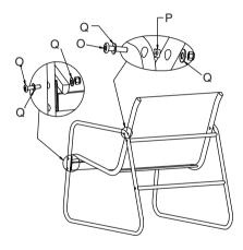
Attention: Washer (Part P) must be put between Leg (Part A) and Seat (Part B).
