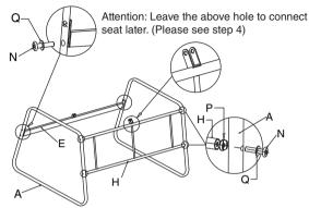
3. Attach the double seat (Part C) to the connecting bar (Part E) using bolt M, washer Q, and nut, as indicated in the diagram.
