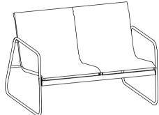
2. Attach the double seat (Part C) to the back frame (Part H) using bolt M, washer Q, and nut, following the diagram.
