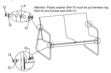
4. Insert surpporting bar (Part F) to double seat (Part C) as shown in diagram.
