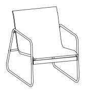
2. Place the single seat (Part B) onto the legs (Part A) as indicated in the diagram, securing it with bolt O, washer Q, plastic washer P, and a nut.
