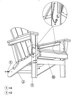
${\bf 5.}$  Assemble holder (part K) by using bolt  ${\rm (}1{\rm)}$  as shown in diagram.
