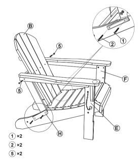
**4.** First, connect the back bar (Part J) with the seat (Part A) using bolt ① as indicated in the diagram.
