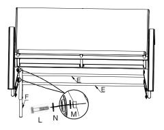
6. Connect the left leg (Part G) to the glider (Part E) using Screw (L), washer (N), and Plastic washer (M) as shown in the diagram.
