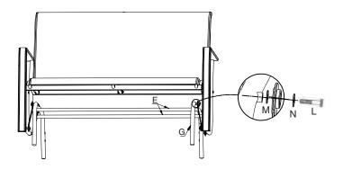
7. Attach the leg connector (Part H) to the legs (Part F and Part G) using Screw (K) as indicated in the diagram.
