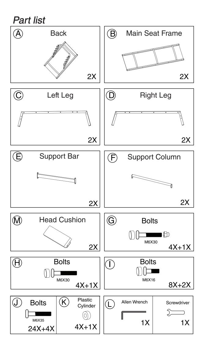
Step 1: Attach the 2 Legs (Parts C and D) to the Support Column (Part F) using Bolt (H) and Bolt (G) as depicted in the diagram.
