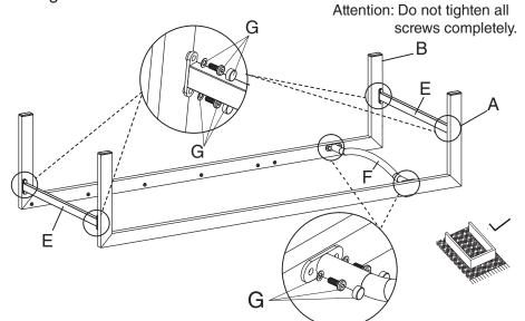
2. Connect Seat(Part C) with Legs(Part A,B)using Screw H.
