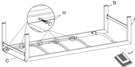
3. Connect Back(Part D) with Legs(Part A,B) using Screw H and Washer K.
