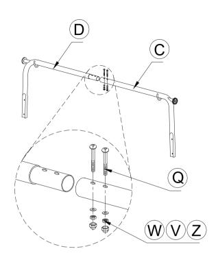
**Step 2:** Connect Part A and Part B with the beam using Bolt U, Washer W, Nut V, and Plastic End-Cap Z as shown in the diagram.
