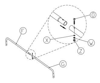
Step 5: Connect the rear foot tube to Part B using Bolt S, Washer X, Nut W, and Plastic End-Cap Z as shown in the diagram.
