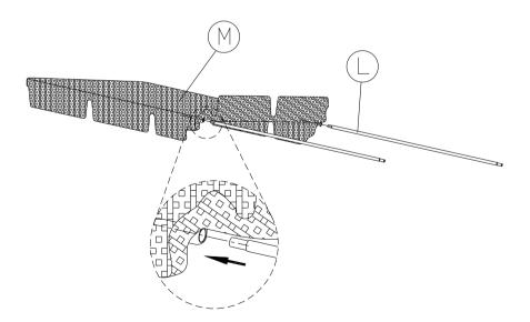
**Step 11:** Connect Part L and Part K to support canopy. Before using, make sure to check that all screws are securely tightened.
