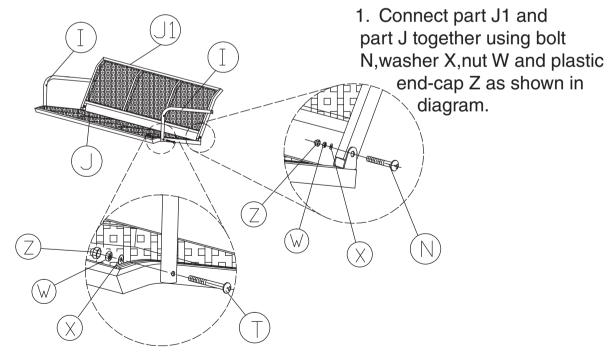
2. Connect part I and part J using bolt T washer X,nut W and plasticend-cap Z as shown in diagram.
