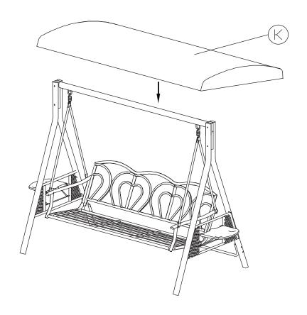
Step 7: Connect canopy with top beam using bolt Y.
