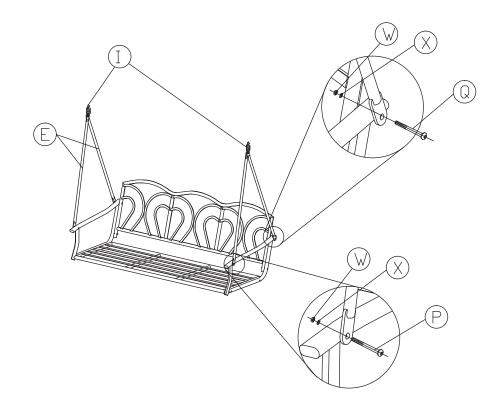
Step 5: Using spring hook (part H) to hook the seat to the frame as shown in diagram.as shown in the diagram.
