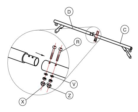
**Step 2:** Connect part A and part B using bolt S washer V, nut X and plastic end-cap Z as shown in diagram.
