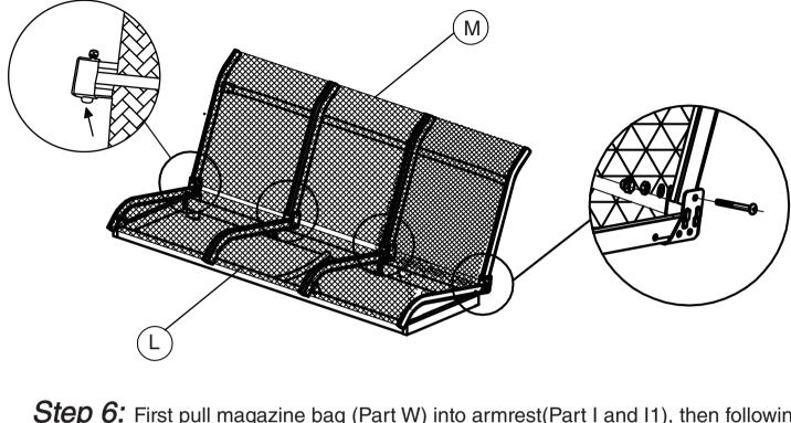
Step 6: First pull magazine bag (Part W) into armrest(Part I and I1), then following below steps to connect nuts.
