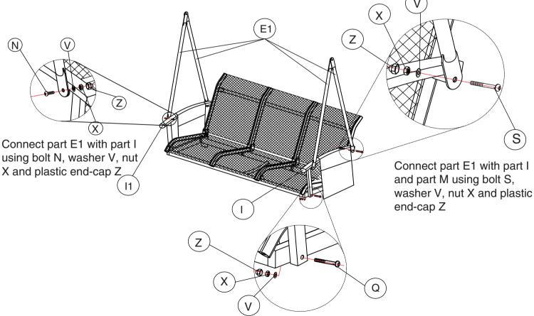
Connect part I with part L using bolt Q, washer V nut X and plastic end-cap Z
