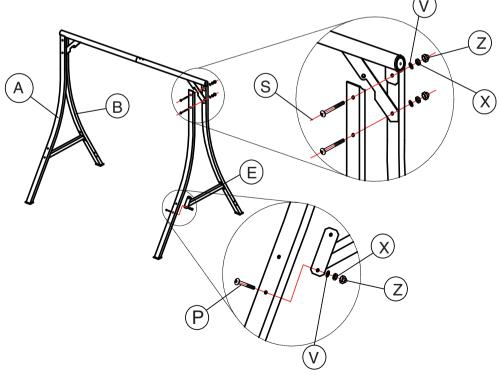
Connect part E and part (A&B) using bolt P washer V, nut X and plastic end-cap Z as shown in diagram.
