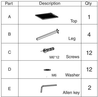
**1.** Connect Top Part (A) and Legs Part (B) using Screws (C) and Washers (D) as shown in the diagram.
