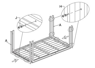
$\mathbf{5.}$  Make sure to check that all bolts are securely tightened before using.
