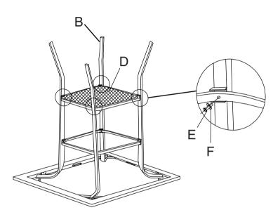
4. Finally, ensure that all screws are securely tightened before using the product on level ground.
