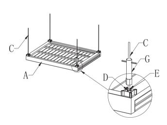
**3.** Position Leg (Part B) to cover Part C, as shown in the diagram. Then, place washer (Part D) and tighten Nut (Part E) to attach Leg (Part B) using Driver (Part G). Finally, cover it with Plastic cap (Part F).
