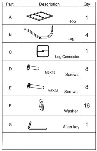
**1.** Connect the top (Part A) and legs (Part B) using Screws (D) and Washers (F) as illustrated in the diagram.
