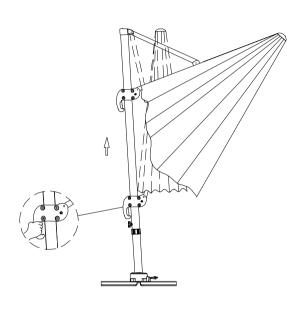
**5.** Attach the crank to the handle. Then, turn the crank clockwise to open the umbrella and counterclockwise to close it, following the diagram.
